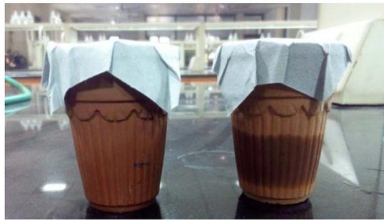
**Fig 5: Silver Earthen Pot for Water Purification**
